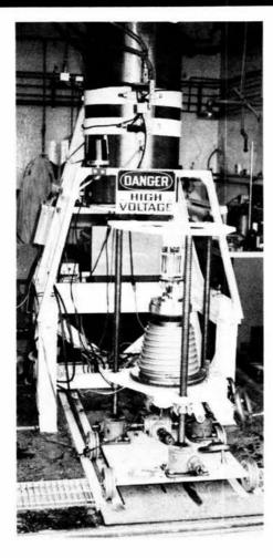
MAGMA SIMULATION FACILITY allowed the first direct measurements of heat transfer rates in a basaltic magma under typical magma chamber conditions.
